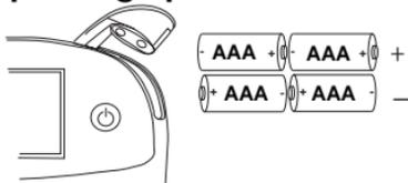
Follow the illustration on the back of the unit when installing the batteries.
