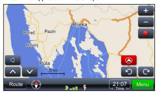
Instant position is determined using a GPS signal – presence of valid GPS signal is marked by the green color of the GPS signal icon
