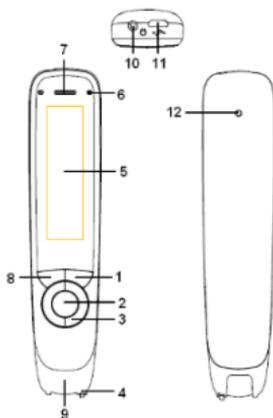
**1. Power On/Off & Back button:** A long press powers the device on or off. In the sub-interface, press this button to exit from the current level back to previous interface. When prompted for selection or input, this button cancels the operation.
