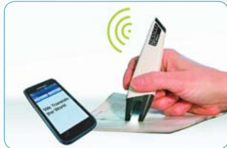
The new Bluetooth design allows on-the-go scanning up to 30 feet from your computer or mobile device. The OCR will transmit any text you swipe directly to your open application. Scanning speed has been increased so you can scan as you read and the recognition will be virtually instant. The new Android compatibility allows users to connect the C-Pen® via Bluetooth to their Android device, scan text, and see it on their mobile devices screen.
