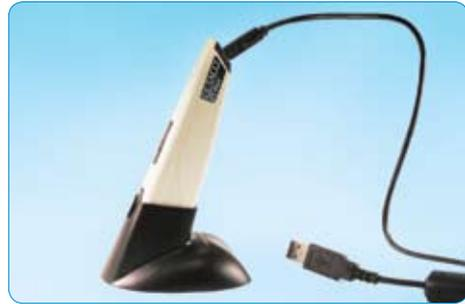
With the ECTACO®/C-Pen® you can scan printed text into your computer to virtually any open application. It connects via USB port and scans 180+ languages. It can also be used as a barcode scanner for inventory management and statistics. The new Google Translate interface now allows you to scan, upload text to your computer, and then translate it to any language via Google Translate.
