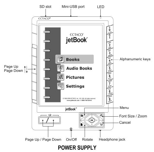
ECTACO® jetBook® is powered by a special Li-ion polymer rechargeable battery.
